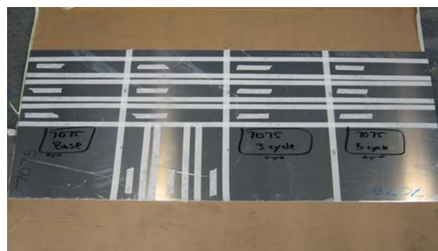
Fig. 3 Marked rectangular samples on uncoated sheet
